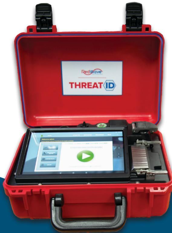
Using proven FTIR technology, it not only identifies solids and liquids, but also gases which pose the greatest danger to responders.
