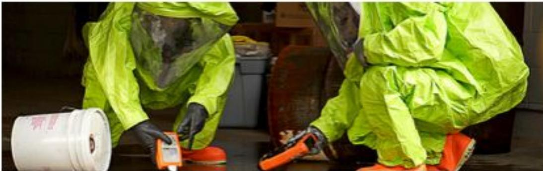
Images above: note that the display screen and the sample sensor (at the bottom of the analyzer) are in the same physical plane, making the act of touching the sample to the unknown substance while manipulating controls and observing the results on the screen difficult. These actions are further complicated by the physical act of kneeling or bending while in gear. Ergonomics are important. [photos from ref. 5,6]
